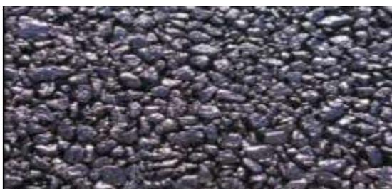
**Gambar 1.** Permukaan Aspal Porous
